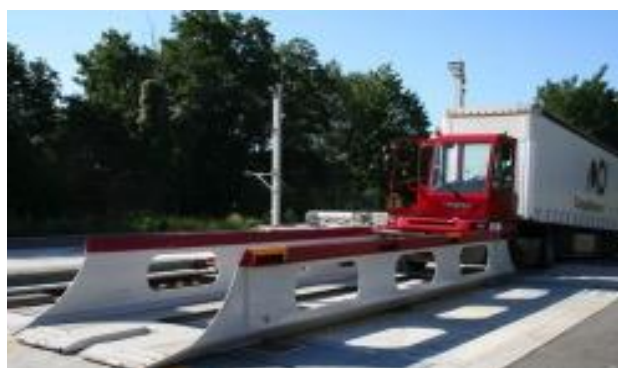
Figure B.6: Fully automatic loading and unloading with CargoBeamer (Source: CargoBeamer AG, 2014)
