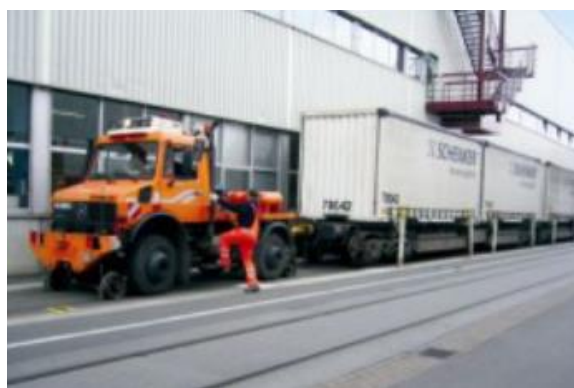
Figure B.8: Combilifter at work (Source: AXIT AG, 2014)
