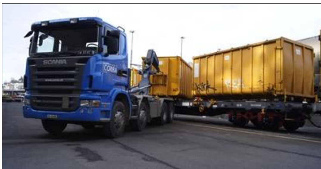
Figure B.4: Roll-off container (Source: Corrà Transporte, 2014)
