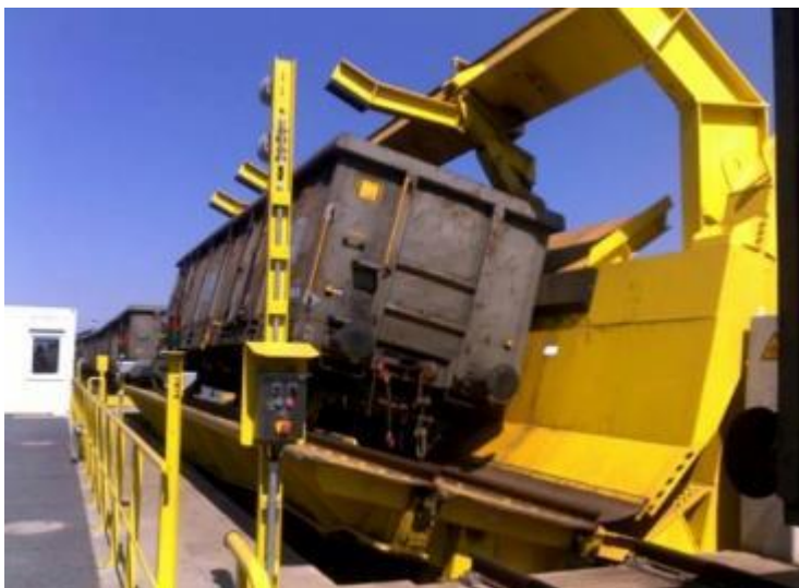
Figure B.13: Wagon tipping system (Source: Badische Stahlwerke GmbH, 2011)
