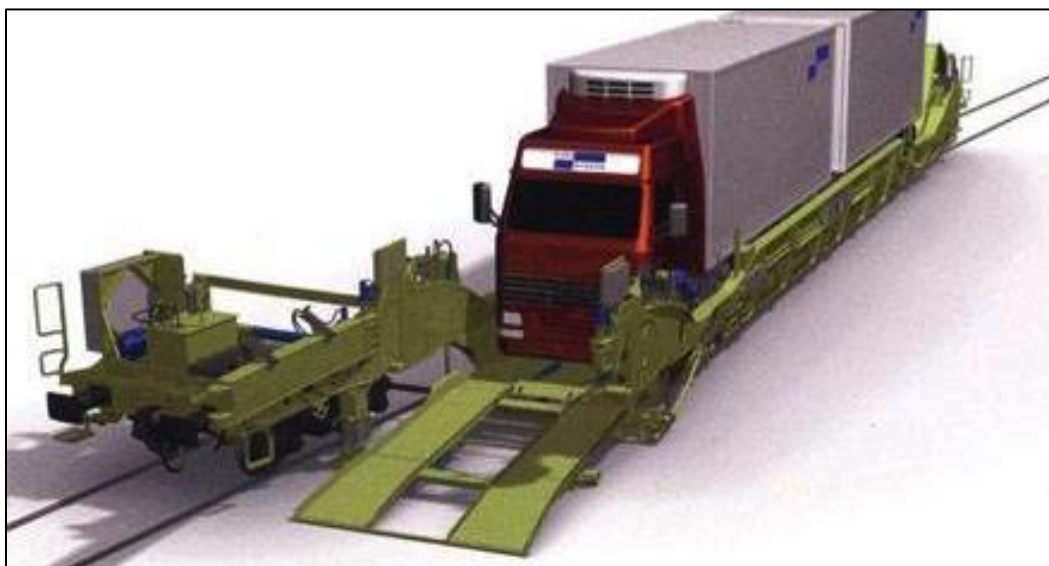
Figure B.10: Flexi-wagon concept (Source: Randelhoff, Flexiwaggon – flexibel ohne Terminals, 2010)
