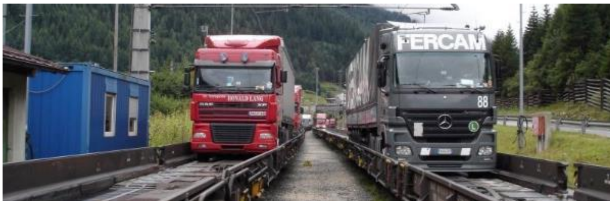
Figure B.5: Loading station of the rolling road (Source: Industriemagazin GmbH, 2009)
