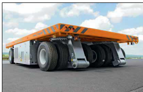
Figure B.3: Left: Platform car; right: selfdriving-platform car (Source: HUBTEX Maschinenbau GmbH & Co. KG, 2014)
