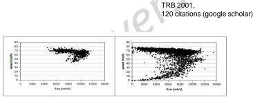
FIGURE 4. Speed-flow relationship on five-lane US freeway; measurement on the left, simulation result on the right.
