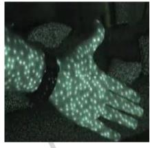
The Underlying Principle 3D Deep Scanning: Structured Light
